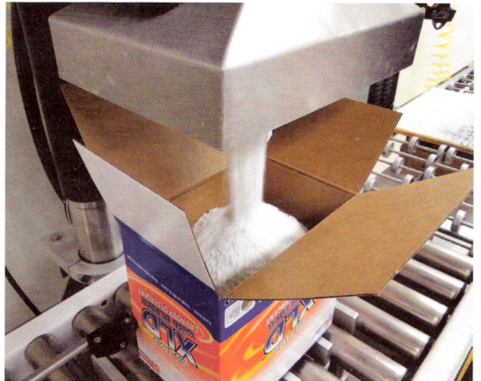
AUDIBLE AUGER. When the 13-lb soap boxes are full, an audible alarm alerts the operator.
